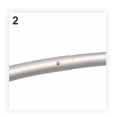
1-2. First join the aluminum tubes to form the support bars of the PopUp: insert each tube in his pair to which he is connected by an elastic, press the button on one of the tubes and push towards the other tube provided with an orifice as shown in Figure 1. When they combine correctly, you will hear a "click" and the button will come out through the hole as in Figure 2.
